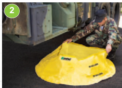
Step 2: Position Pool underneath spill source.
